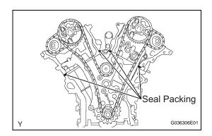
(c) Apply continuous beads of seal packing (diameter 3 to 4 mm (0.12 to 0.16 in.)) to the 4 locations shown in the illustration.
