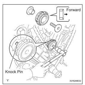
(b) Temporarily install the No. 1 idle gear shaft together with the No. 2 idle gear shaft with the knock pin of the No. 1 idle gear shaft and the knock pin groove of the cylinder block are aligned.
