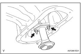
(c) Apply a continuous bead of seal packing (diameter 3 to 4 mm (0.12 to 0.16 in.)) to the oil pan as shown in the illustration.
