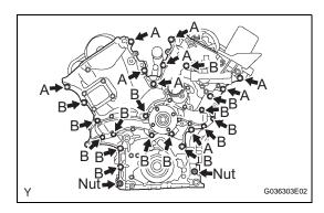
(g) Install the timing chain cover with the 24 bolts and 2 nuts. Tighten the bolts and nuts uniformly in several steps.
